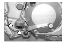
• Remove the return spring of the rear brake pedal.
