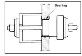
• Fit the specified crankcase bearings to the special tool.
