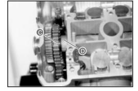
Temporarily fit no. 2 valve motion idler gear/sprocket 1 with copper washer 3 and thrust washer 2.
