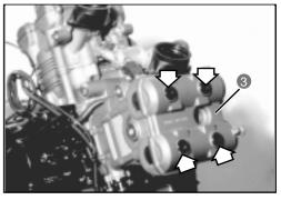
• Turn the crankshaft until the "F|T" line on the generator rotor is aligned with the mark on the valve gear timing inspection hole, and bring the camshafts to the position shown in the figure.
