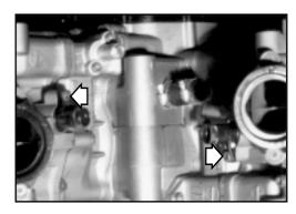
• Install the thermostat casing with the coolant lines and firmly tighten the fastening screws.
