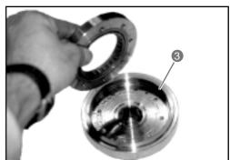
When fitting starter coupling housing 3 on the generator rotor, align hole B in the starter coupling housing with projection C on the generator rotor.
