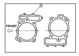
• Fit dowel pins 2 and new gaskets 3 to the crankcase.
