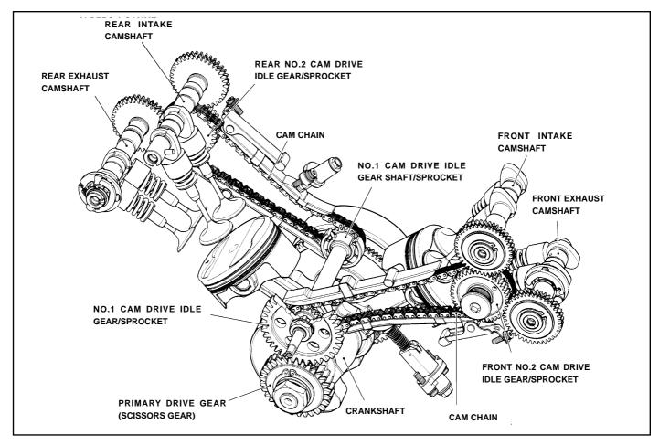
In this system, the angular position of the sprocket teeth on the no. 1 valve motion idler gear/sprocket relative to the primary driving gear varies between the compression and exhaust top dead centres.
