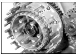
• Unlock clutch drum nut 8.
