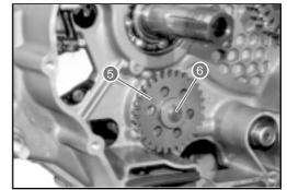
• Fit the thrust washer on the countershaft.
