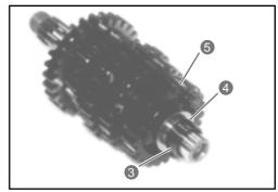
• Remove the circlip using the specially designed tool.
