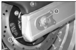
• Count 21 pins (20 pitches) of the chain and measure the distance between the two points. If the distance exceeds the operating limits, the chain must be substituted.
