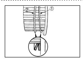
Insert the clutch driving and driven plates one by one into the clutch drum in the order shown in the figure. Insert no.2 driving plate B first. (There are two types of driving plates, no. 1 and no. 2, differing in inside diameter.)
