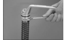
Seal the fork by tightening the support tube plug to the correct torque.
