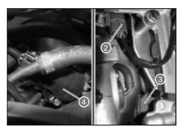
Connect the suction tube from the rear butterfly body to the secondary air valve and the relative sleeves.
