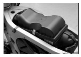
Carefully eliminate dust and dirt from the filter element by using compressed air.
