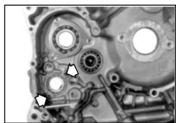
• Remove bearings 1, 2, 3, 4, 5 and 6 using the special tools.
