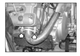
• After removing the screws as indicated in the figure, remove the rear cylinder exhaust tube.
