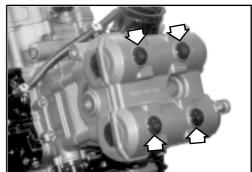
• Tighten tappet inspection hole plug 2 and generator cover plug 3 with the specified torques.
