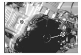
• Fit new O-rings to the cooling system joint and grease them.
