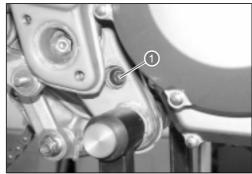
• Unscrew the nut **2** and extract the fixing pin that fixes the engine to the frame.
