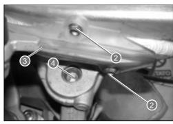
The spindle 4 relative to the fixing nut of the connection rod to the frame is therefore left free.
