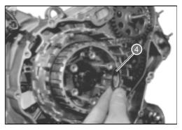
• Tighten clutch drum nut **5** with the specified torque using the specially designed tool.
