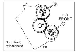
• Remove camshaft bearings 4 after unscrewing the bolts.
