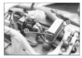
Apply 12 volts to the terminals **A** and **B** and check the continuity.
