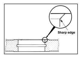
• Insert the bearings installed in the special tool into the crankcase half as shown in the figure.
