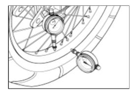
Bearing wear generally causes an excessive axial movement or eccentricity.
