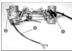
• Remove the fuel feed tubing 1 by removing the nuts.
