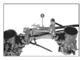
• Remove the fuel pressure adjuster 2 and the incoming fuel tube union 3 from the fuel feed tubing.
