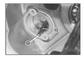
• While holding the generator rotor with a 36-mm spanner, remove no. 1 valve motion idler gear/sprocket nut 3 and the related washer.
