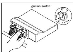
• Do not connect the battery with inverted polarities. This will instantly damage components of the FI system when the circuit is switched on.
