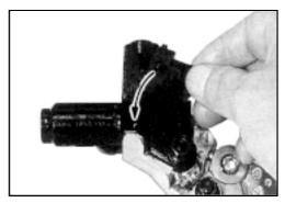
• When reassembling the brake pump onto the handlebars, tighten the upper fixing bolt first.
