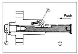
• From this position, unscrew adjuster bolt 1 until adjuster rod 2 locks. The timing chain tension adjuster is now ready for installation.
