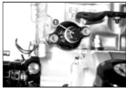
• Tighten adjuster bolt 1 with the specified torque.
