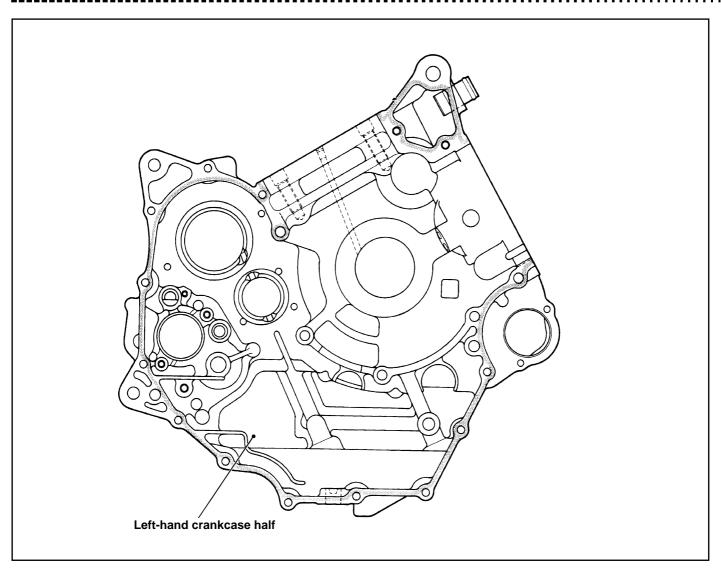
When fastening the left and right crankcase halves, tighten each bolt gradually to equalize the pressure. Tighten all fastening bolts with the specified torques.
