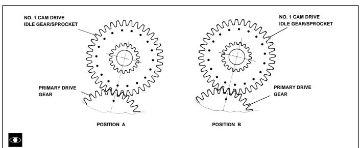
The no. 1 valve motion idler gear/sprocket has in fact only one punched mark. This mark should be located in either of the two positions illustrated, as is appropriate for their respective top dead centres.
