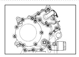
• Fit starting idler gear 1, spacer 2 and shaft 3.
