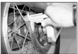
Carry out the distortion check of the disc utilising a comparator with the disc mounted on the hub.
