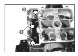
• Remove cylinder head nuts (M6) 4.
