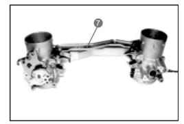
• Remove the N° 1 throttle lever 1 and the N° 2 throttle lever 2. Remove the connection rod 3 by unscrewing the nuts.
