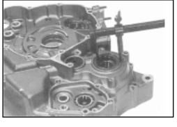
• Remove the oil jet from the left crankcase half.
