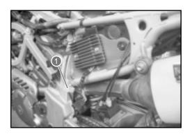
If the peak voltage at the lead coupling of the crankshaft position sensor is normal, but the peak voltage at the lead coupling of the ECM CPU is abnormal, the wiring must be substituted. If both peak voltages are abnormal, substitute the crankshaft position sensor and carry out the test again.
