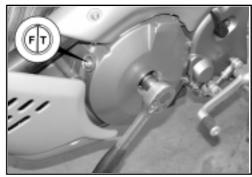
• To check the valve tappet clearances of the N° 1 cylinder (front), insert a feeler gauge between the valve stem and the cam. If the clearance is not correct, adjust it within the specified range.
