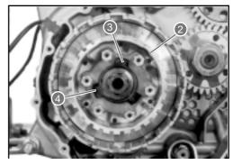
• Remove driving cam 3 and driven cam 4 from clutch drum 2.
