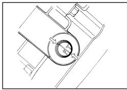
When checking the position of the no. 2 valve motion idler gear/sprocket, take up the timing chain slack on the side of chain guide 2 by holding the no. 2 valve motion idler gear/sprocket with one hand.
