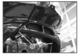
• Disconnect the indicator connectors. One is indicated in the figure and the other is on the opposite side of the machine.
