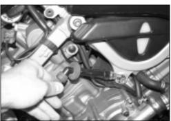
Test the peak voltage of the primary winding of the N° 1 ignition coil using the following procedure.
