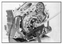
• Lock clutch drum nut 5 with a punch.
