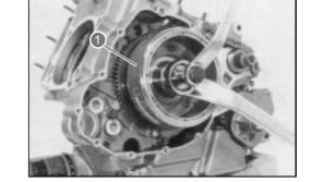
• Remove key 2 and starting driven gear 3.
