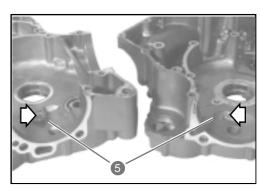
• Remove the oil seals using the specially designed tool.
