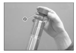
Check that the internal surface of the sheath and external surface of the stem are in good condition.
