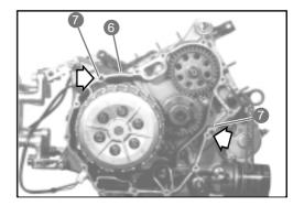
• While holding the generator rotor with a 36 mm (1.417 in) spanner, remove the bolts fastening the clutch springs and then the spring following a crosswise pattern.
