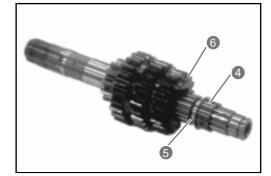
• Remove the circlip using the specially designed tool.
