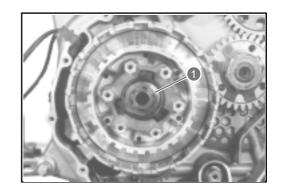
Remove clutch drum 2 together with driving cam 3 and driven cam
