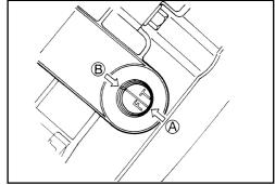
• Apply molybdenum bisulphide grease to the no. 2 valve motion idler gear/sprocket, to its shaft **1** and to thrust washer **2**.
