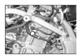
• Remove the secondary air tubes from the cylinder by unscrewing the two relative screws (for each tube) as indicated in the figure.
