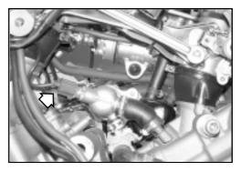
• Remove the connector of the camshaft position sensor.
