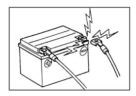
Before measuring the voltage on any terminal of the electrical system, check that the voltage of the battery is 11V higher. Terminal checks carried out with an insufficient battery voltage can cause diagnostic errors.
