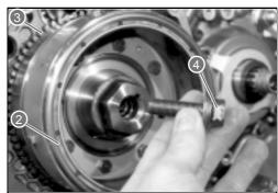
• While holding the generator rotor with a 36-mm spanner, tighten its bolt 4 with the specified torque.
