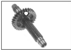
• Remove 2nd drive gear 3, its bushing 4, and washer 5.
