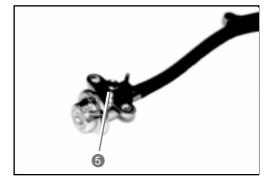
• Replace the fuel pressure adjuster on the fuel feed tubing.
