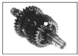
• Remove 4th driven gear 6 and its bushing 7.
