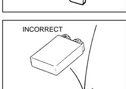
• Take care to not touch the electrical terminals of the ECM. The static electricity of the body can damage the component.
