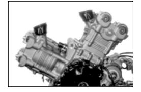
• Install camshaft position sensor 1 and tighten the fastening bolts with the specified torque.
