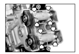
• Tighten the camshaft bearing bolts with the prescribed torque.
