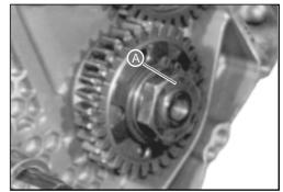
• While holding the generator rotor with a 36-mm spanner, tighten the primary driving gear nut with the specified torque.
