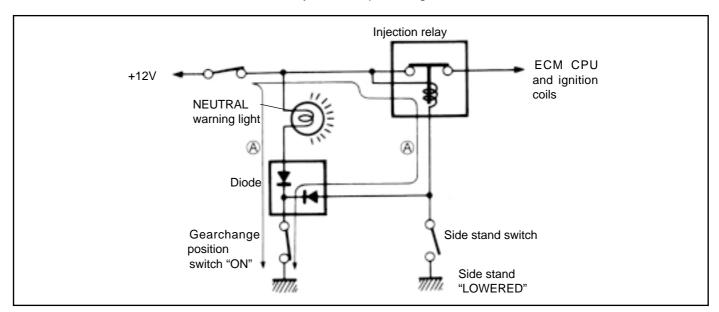
2. Gearchange: "GEAR INSERTED (OFF)" / "Side stand raised (ON)"
