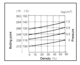
Fig. 2 Boiling point - engine coolant density curve.
