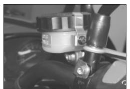
• Remove the fluid chamber along with the tube connector by releasing the elastic ring **3**.
