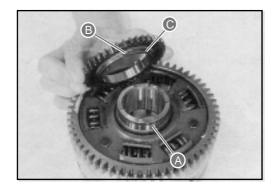
• Fit clutch driven cam 5 on clutch drum 6.
