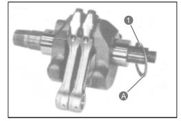
• Fit the crankshaft in the left crankcase half.
