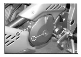
Turn the engine camshaft to bring the piston of the N° 1 cylinder (front) to the top dead centre (T.D.C.) position of the compression cycle. Align the "F/T" line on the generator rotor with the timing inspection hole line and bring the camshafts to the indicated position in page B- 10.)
