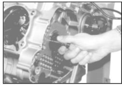
• Fit a new O-ring in engine sprocket spacer 1.
