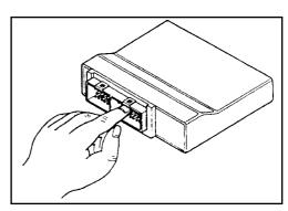
Before connecting or disconnecting an ECM coupling, make sure that the ignition switch is in the OFF position. This will prevent damage to the electronic parts.
