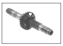
• Remove 5th driving gear 7 and its bushing 8.
