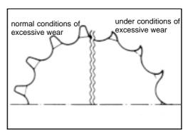
If excessive wear is noted, substitute the various components.
