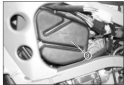
• Remove the filter compartment by loosening the two fasteners on the butterfly body as indicated in the figure.
