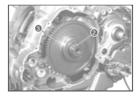
Remove no. 1 valve motion idler gear/sprocket 4 and timing chain
