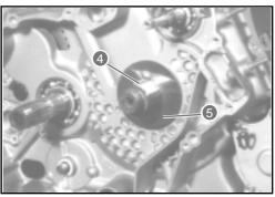
• While holding the generator rotor with a 36 mm (1.417 in) spanner, remove its bolt and washer.
