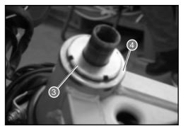
Check the condition of the various parts removed. If necessary, substitute the steering bearings. Remove the bearing seats using a mallet and a drift as shown in the figure.
