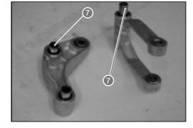
Remove the oil seals. Using a drift of the correct diameter, knock out the roller bearing from its seat, exerting pressure on the external diameter of the bearing.
