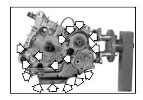
• Separate the crankcase into two parts, left and right, using the specially designed tool.
