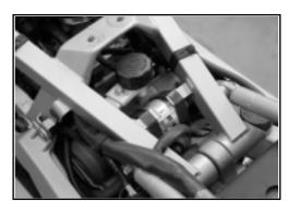
• Remove the rear cylinder head valve cover by unscrewing the four relative screws shown in the figure.
