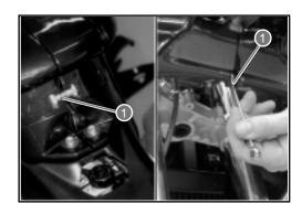
• Finally, remove the two fixing screws 2. Disconnect the overflow tube from the left fuel tank.
