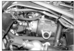
• Unscrew the screws 3 and free the choke adjuster support plate.
