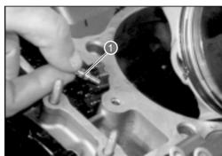
Apply a film of specific product to the mating surfaces of the left and right crankcase halves as shown in the figure.
