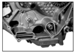
• Fit washer **3**, pin **4**, oil pump driven gear **5**, and circlip **6** to the oil pump shaft.
