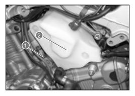
• Loosen the two fasteners on the collectors.
