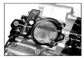
Place a clean rag over the cylinder base to prevent the piston pin circlip from falling into the crankcase.
