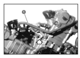
• Fit the spark plugs on each cylinder head and tighten them with the specified torque.
