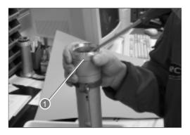
Using a wide screwdriver, exert pressure under the sealing ring and at the same time, rotate the sliding section to allow the sealing ring to slide out. Pull out the plate that is underneath the sealing ring.
