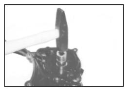
• Fit a new oil seal into the clutch cover using a suitable tool.
