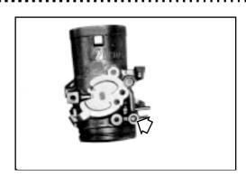
• Remove the air screw with the spring, washer and O-ring.
