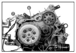
• Grease the oil seal rim on the clutch cover.
