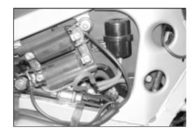
• Disconnect the incoming fuel tube by unscrewing the union fasteners as shown in the figure.
