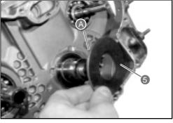
• Fully insert key 6 into its slot on the crankshaft.
