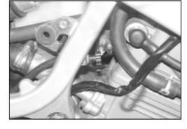
• Replace the complete T-shaped coil support.
