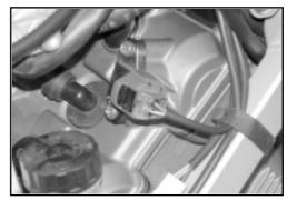
Remove the radiator by unscrewing the three screws 3 as shown in the figure and lift it up to remove it from its supports.
