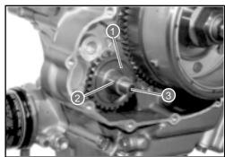
• Fit bushings 4 into the crankcase and the generator cover.
