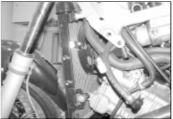
• After reassembling the radiator, make sure that the engine coolant is topped up in the radiator (see page B-20 for further information on topping up).
