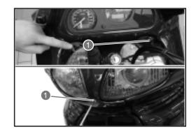
Remove the front protection by unscrewing the two lower screws
