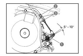
• Fully screw in throw-out **4** onto the throw-out lever and place both parts on the push rod.
