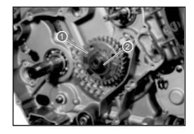
• Fit the primary driving gear nut.
