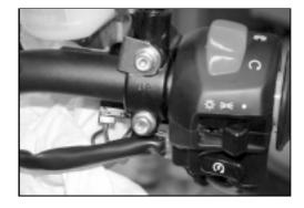
Place a cloth underneath the brake pump joint bolt to collect the last drops of fluid left in the system. Remove the joint bolt 1 and disconnect the brake tube.
