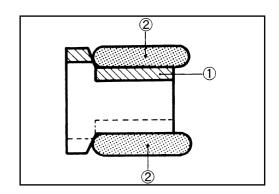
• Position the end gaps of the three piston rings as shown in the figure. Before inserting the pistons into the cylinders, ensure that the ring end gaps are positioned as indicated.
