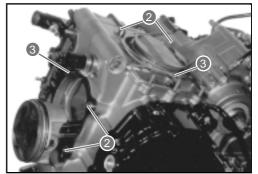
Apply engine oil to the sliding surfaces of the pistons and cylinders.
