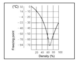
Fig. 1 Freezing point - engine coolant density curve
